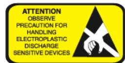
These products are sensitive to electrostatic discharge and should not be handled except at a static free workstation. Take precautions to prevent ESD; use wrist straps, grounded work surfaces and recognized anti-static techniques when handling the IC.
