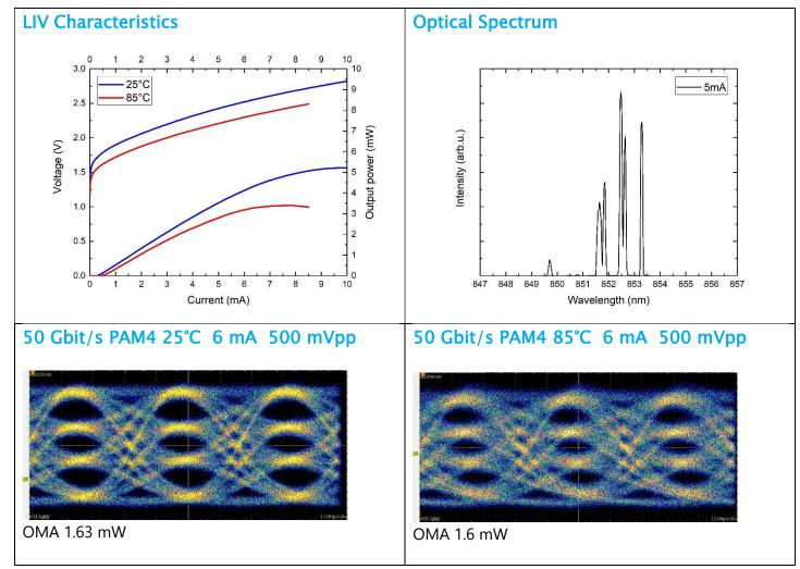
Transmitter: SHF BPG 12104A. Receiver: Tektronix DSA8300 w. 80C15 Optical Sampling Module.
