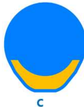
Contact shape Active area: 24 \mu\text{m} diameter, \sim 455 \mu\text{m}^2
